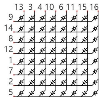
Connection mode of Common Cathode
