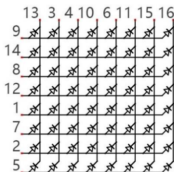
Connection mode of Common Anode
