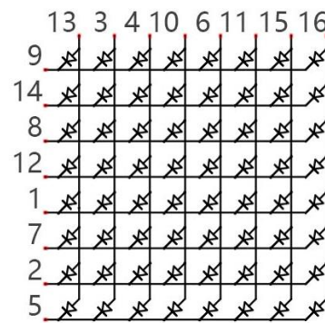
Connection mode of common cathode
